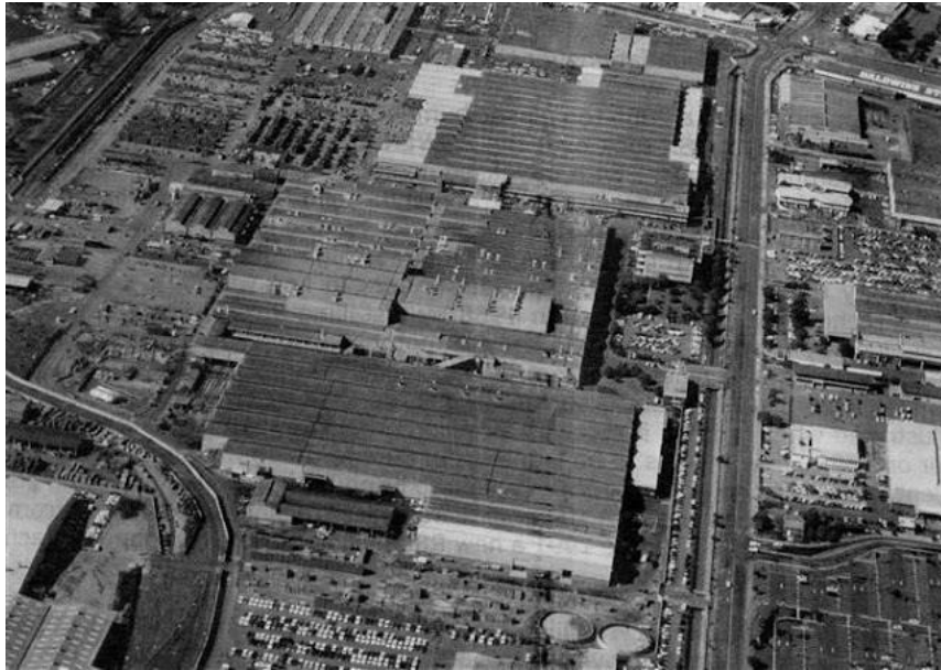
An aerial view of the new Motor Assemblies plant at Prospecton in the 1990s. The body shop is in the foreground, the paint shop next, and then the vehicle assembly shop. Beyond that is the engine machining and assembly shop and on its right is the trim shop. Prospecton Road runs next to these buildings and to the right is the Product Engineering Centre and the training school.
