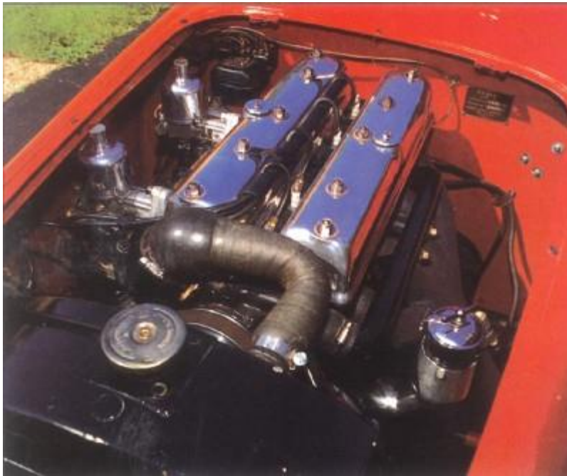
The 1950 Healey Silverstone was powered by a 2.5 litre four-cylinder engine.
