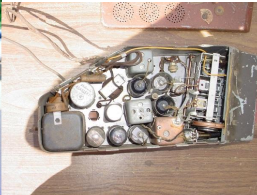
INNER WORKINGS OF THE SAME CAR RADIO
