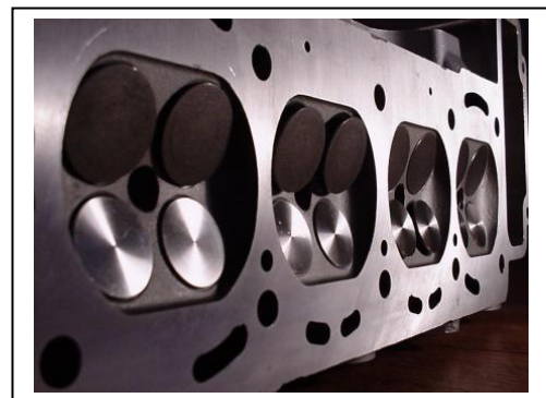
Triumph Dolomite and single cam 16 valve aluminium head
