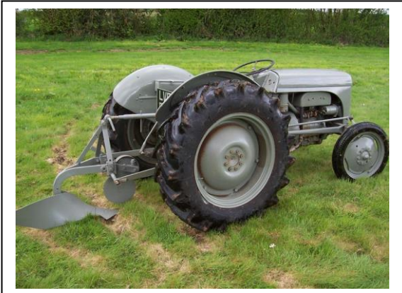
Ferguson TE fitted with hydraulic third bar stabiliser for ploughing.
