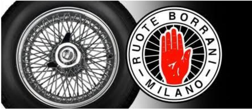
Carlo Borrani was actually born in California but started up a new company with a partner in Milan using the patented Rudge-Whitworth design of a tapered splined hub to which a tapered wheel's centre could swiftly be fitted and locked into position by means of a single wheel nut or a knockoff. As you know, one uses a suitable hammer to tighten or loosen the knock-off.
